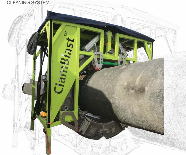
SeriBlast<sup>TM</sup> uses fully automated closed cycle abrasive blasting technology to cost effectively resolve the issues of manual open blasting by reduced manning andreduced environmental impact and significantly reducing consumption of abrasives.
